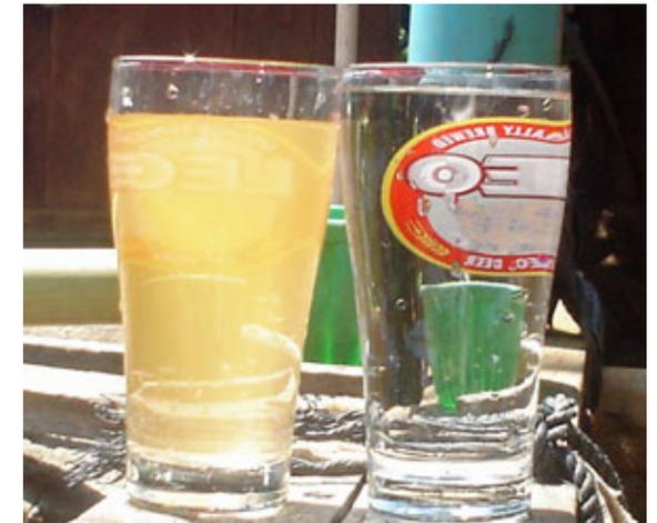
The water in the glass on the left comes directly from the water available from the water pipes in the bateyes. On the right is the same water after it has passed through a bio-sand filter.
